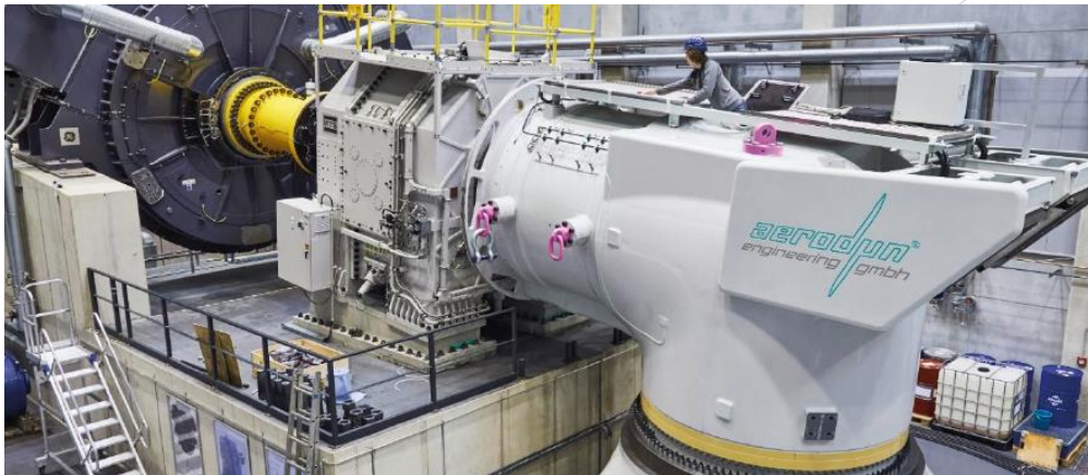
Figure 12 Test of the drive train under torque and bending load. Blue part in the background: E-motor to generate the torque load. Yellow part: torque coupling. Grey box with angled top: device to apply bending moments, [9].
