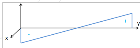
Figure 16 Bending moment over free length of Flexpin (vertical axis) vs. length / y-coordinate.
