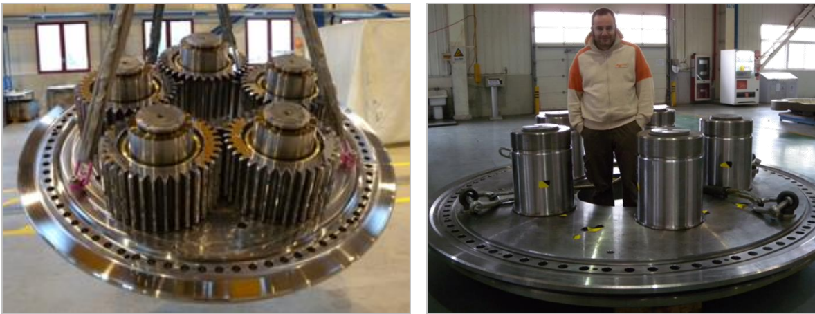
Figure 4 Left: Single-wall planet carrier (large circular plate) with five Flexpins and spur planetary gears assembled, for a 3MW MGB. Right: Upscaled version, bearings and planet gears not yet mounted onto the Flexpins. Planets and bearings not yet assembled, for a 6MW MGB.
