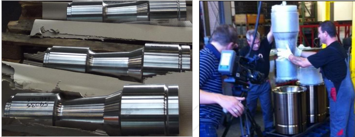
Figure 8 Left: Flexpin pins, awaiting transport to heat treatment. Right pin is cooled down and inserted into sleeve.
