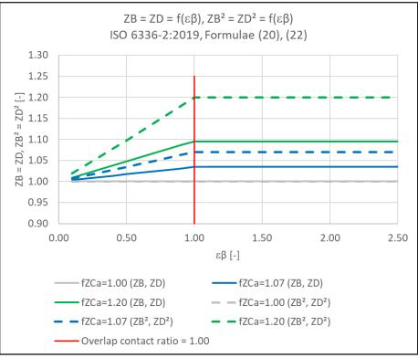
Figure 2 Zone factors  $Z_{KH\beta-C}$  B and  $Z_D$  and their square as a function of  $f_{CZa}$  and overlap contact ratio  $\varepsilon_{\beta}$ .
