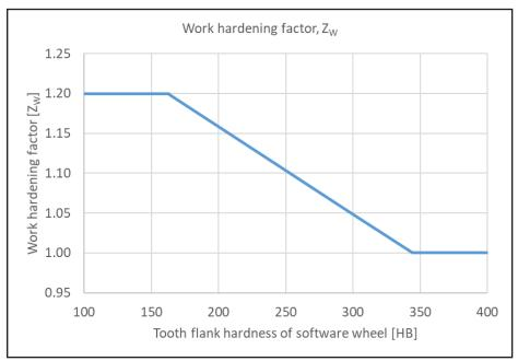
Table 7Work hardening factor  $Z_W$ , ISO 6336-2:2019, for combination of surface-hardened steel<br/>pinion with ductile iron gear.
