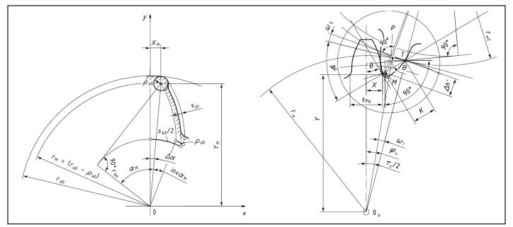
Figure 4 Left: Quantities at the shaper cutter, (Ref. 6). Right: External gear in mesh with shaper cutter, coordinates X and Y of tangent point, tangent angle  $\theta$  and tooth thickness  $s_{Fnr}$  (Ref. 6). Tooth root fillet radius  $\rho_F$  and the bending moment arm  $h_{F\theta}$  not shown explicitly.
