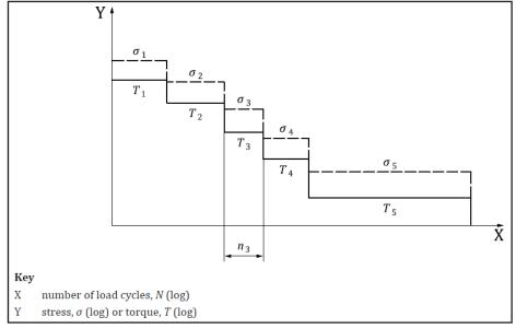
Figure 6 Load and stress spectrum, Figure 2 in ISO 6336-6:2019. The figure explains how the load (torque) spectrum, represented by the torque levels  $T_i$ , associated with a speed level ni each, is converted to a stress spectrum with stress levels  $\sigma_i$  (for speed levels  $n_i$ ), using the methods given in ISO 6336-2 and -3. Above and below figures were combined in one figure in 2006 edition, lacking some clarity.
