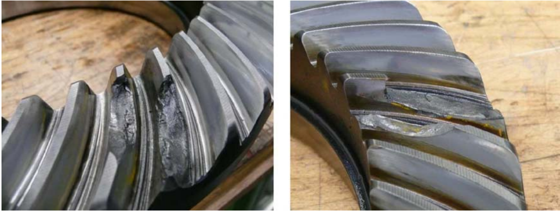
Figure 2. Flank breakage on two different wheels
