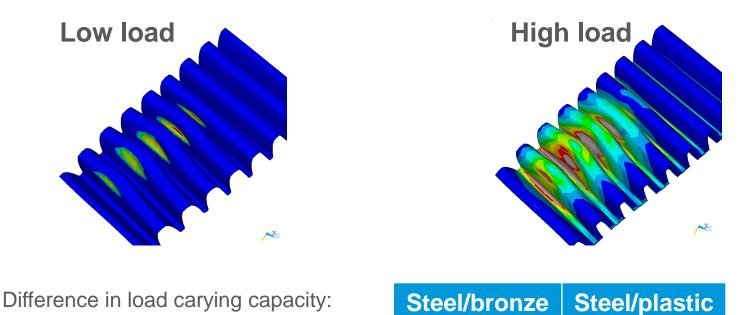
\*Due to running in, flank pressure lowers and conditions become similar to globoidal worm gears
