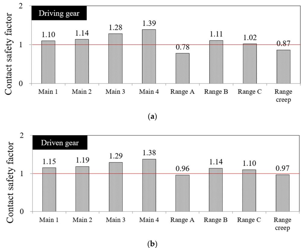
**Figure 8.** Results of contact safety factor for gears of the 86 kW class agricultural tractor transmission used in this study: (a) driving gears; (b) driven gears.
