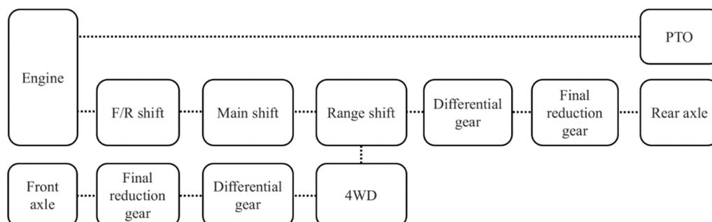
**Figure 4.** Power flow of the 86 kW class agricultural tractor used in this study.
