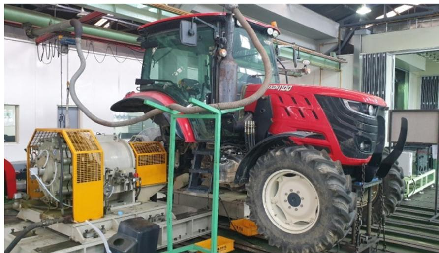
**Figure 6.** A photo of the axle dynamometer test bench used in this study.
