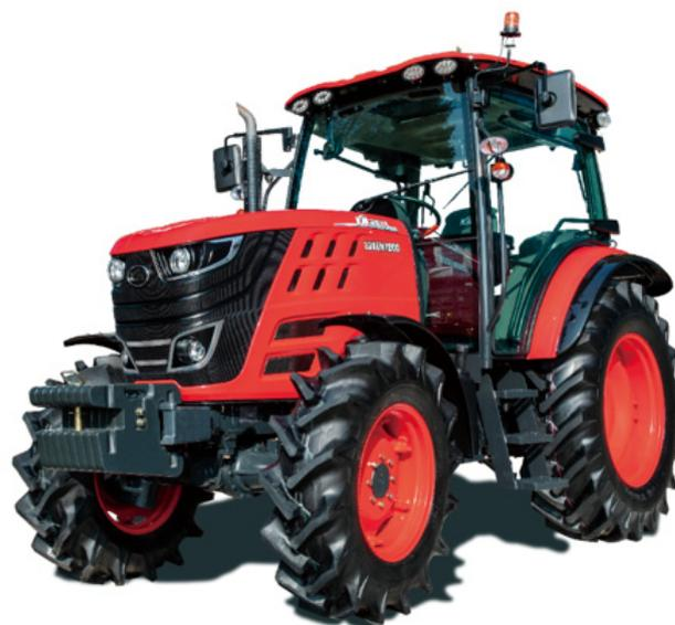
**Figure 1.** The 86 kW class agricultural tractor for the field test used in this study.
