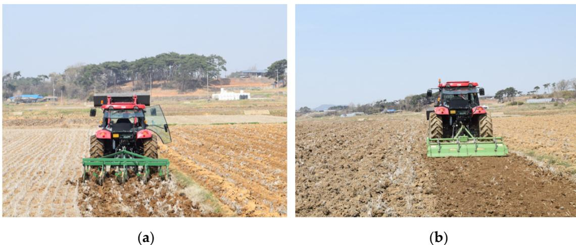
**Figure 2.** Photos of the 86 kW class agricultural tractor during the field test: (a) plow tillage; (b) rotary tillage.
