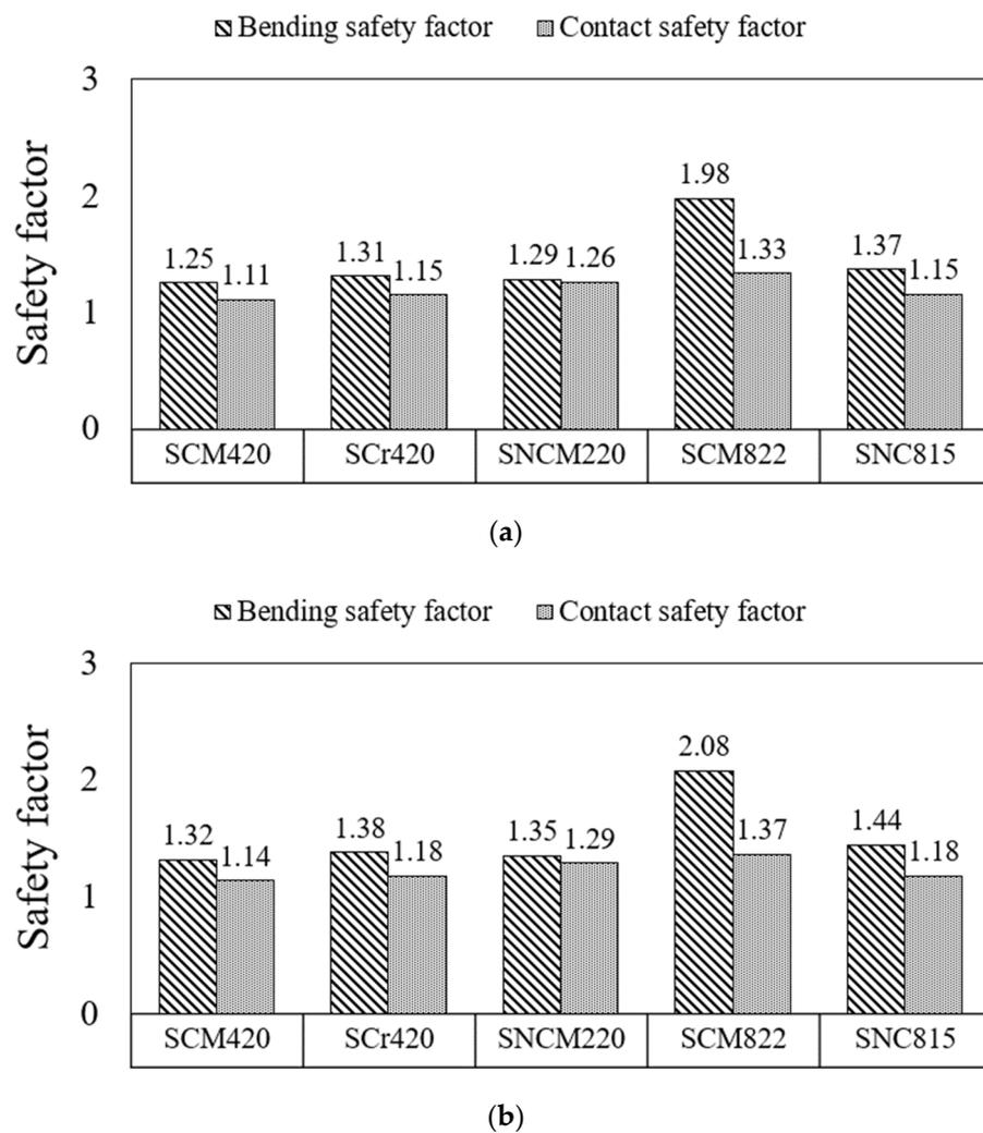
**Figure 10.** Results of safety factor analyses for the range shift B gears with different materials: (a) driving gear; (b) driven gear.
