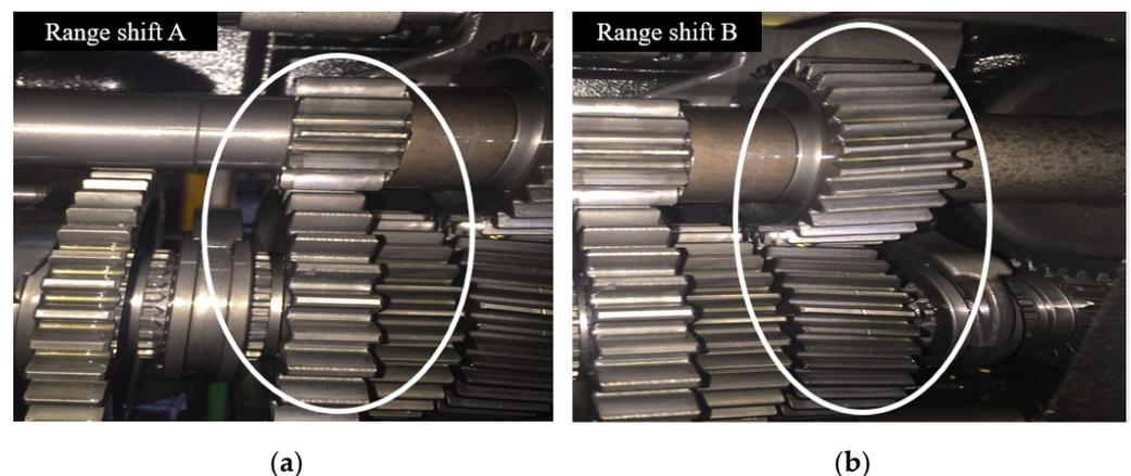
**Figure 11.** Results of the dynamometer test for the range shift gears: (a) range shift A gears; (b) range shift B gears.
