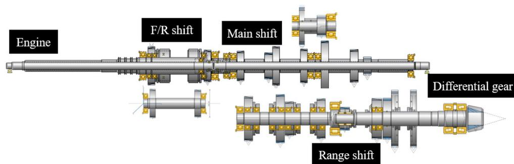
**Figure 5.** Simulation model of the 86 kW class agricultural tractor transmission developed in this study.
