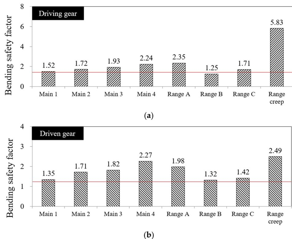
**Figure 7.** Results of bending safety factor for gears of the 86 kW class agricultural tractor transmission used in this study: (a) driving gears; (b) driven gears.
