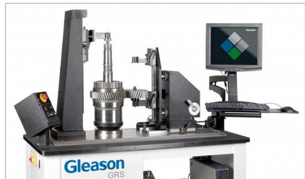
Preferably, the use of existing master gears is targeted. The master gears can be entered in KISSsoft and the rolling with the production gear can be analyzed. The roll testing can be done on a Gleason roll testing machine.
