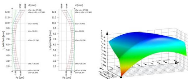
The modifications and tolerance ranges for profile and lead are displayed in K-diagrams. Combined modifications are displayed in detailed 3D graphics.
