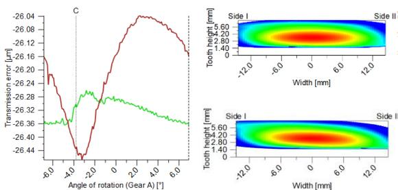
The loaded tooth contact analysis shows the behavior under load, such as stress distribution and contact pattern. The transmission error (PSTE) is used to analyze the noise excitation of gears.
