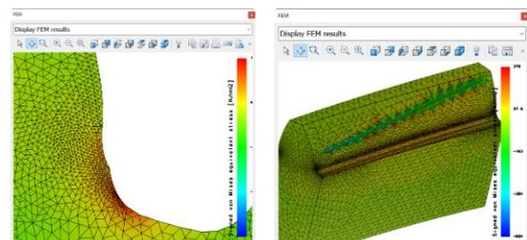
A 2D FEM calculation is sufficient to determine the tooth root stress caused by grinding notches. A 3D
