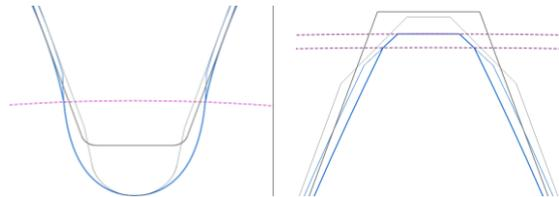
Creating a gear chamfer during premanufacturing requires a separate tool. The angle and size of tooth tip chamfer can be defined in KISSsoft based on the required tip form circle, considering different tolerance conditions.
