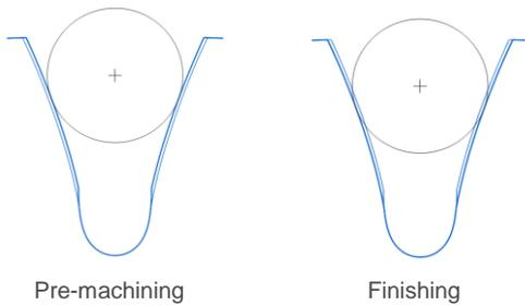
A flattened measuring ball can be defined for spline profiles, to prevent the tooth root from being touched. In the case of deep tooth forms, the ball or roller diameter is automatically calculated to take a correct measurement outside the tip circle.
