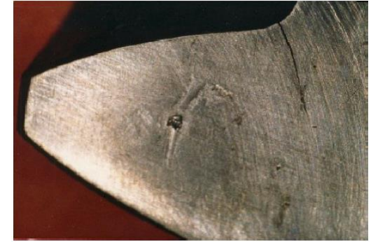
Figure 43 - Bending fatigue crack
