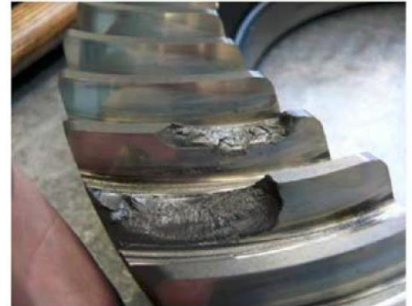
Figure 1 Flank breakage and pitting on wheel.
