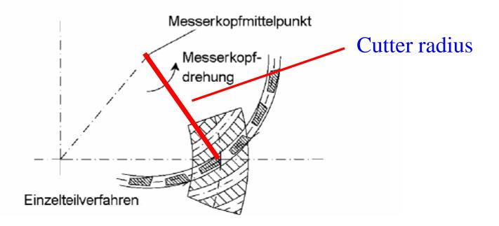
The workpiece has no rotation while the cutting tool plunges.
