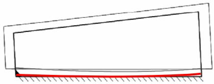
Face Milling requires bigger tilting of the cutterhead in order to create the required lengthwise crowning.
