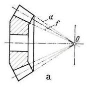
Face Milling (single indexing) modified tooth height
