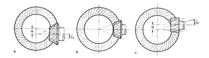
Hypoid gears have an offset between the axes.
