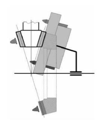
Bevel gears with ratio > 2.5, the ring gear usually is form cut (FORMATE, NON-GENERATED)
