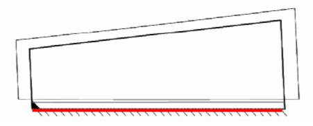
Face hobbing requires only little tilting of the cutterhead in order to create the required lengthwise crowning. Cyclopalloid doesn't apply tilt at all.
