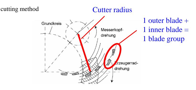
The workpiece rotates continuously while the cutting tool plunges. The effective curvature radius is influenced by the number of blade groups and cutter radius.
