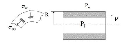
Stresses on the inner edge of the hub (outer part) critical
