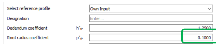
Figure 6.1-2 Change root rounding factor for sun, planet and ring gear to 0.10.
