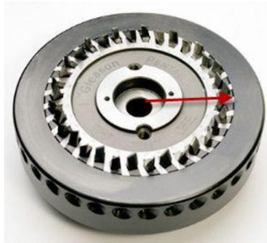
Figure 3.2-1 Face Hobbing cutter head. Radius is defined from center to the cutting edge of the blade.
